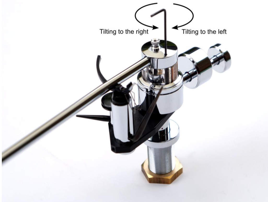
Fig. 1. The hexagon key, going through the armtube flange, is ready to turn the pivot up or down.
